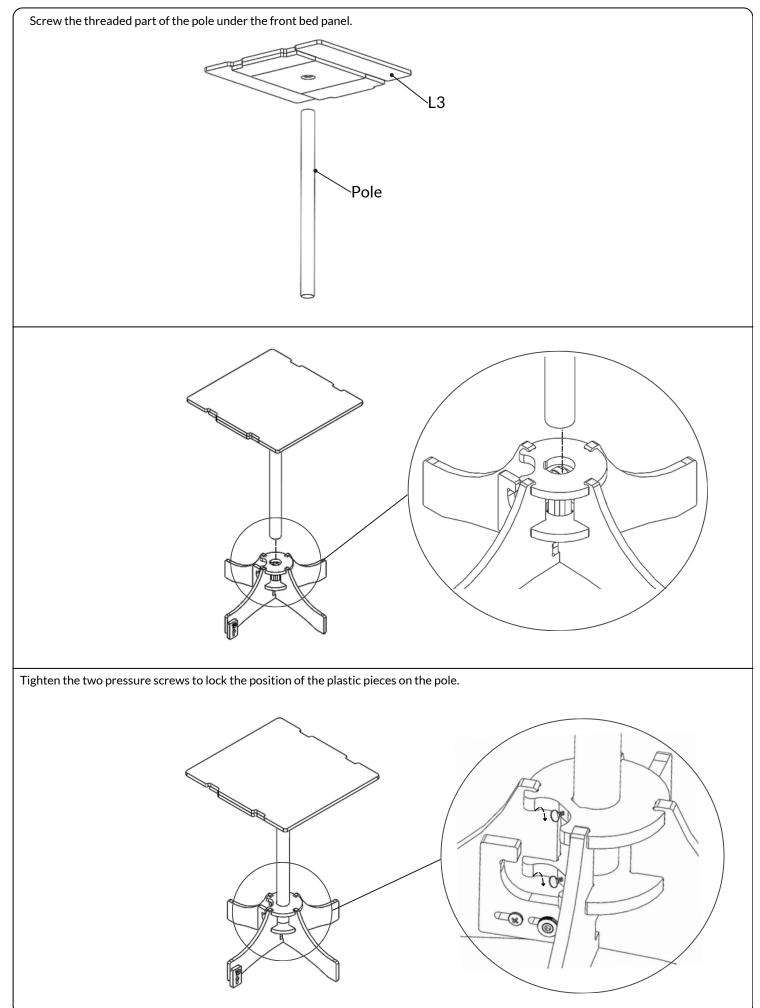
Loosen the wing nut slightly to release the lock.
