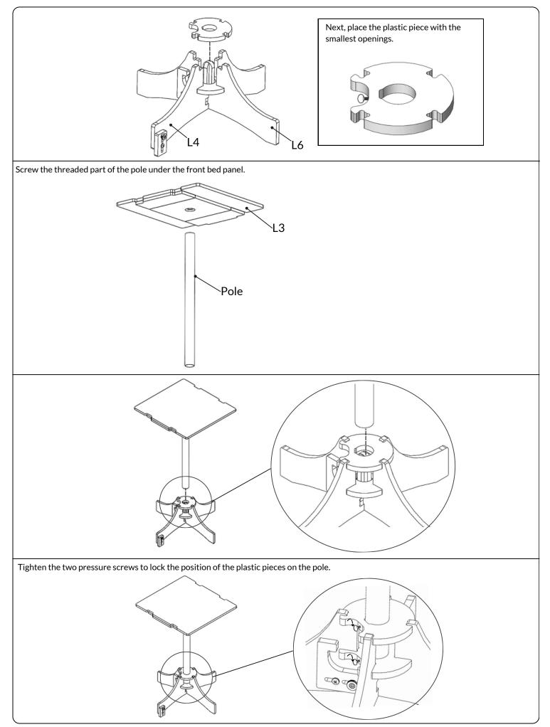
Move the lock towards the table pole and tighten the
