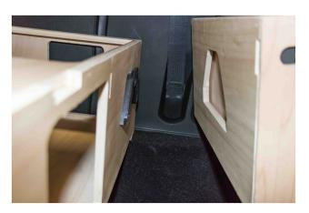
3. Insert the two kitchen drawers (sink drawer and burner drawer) in the fastening system of the central module.
