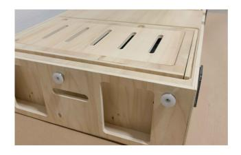
6. Insert the leveling pads on the central box. Refer to the parts list section to identify the number and location of short and long pads according to your vehicle model.
