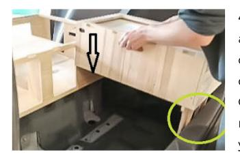
4. Adjust the position of the central module and kitchen drawers so that they are as close as possible to the opening of the trunk door. Make sure that the legs are straight. Caution: always move the boxes (central module AND kitchen boxes) together when you adjust their position.
