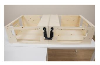
5. Screw the U-bracket into the center module inserts. Screw from the inside and use a screw and a washer per hole.
