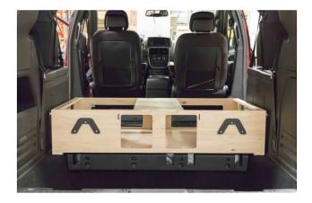
2. Insert the central module into the vehicle and place it in the center of the space.
