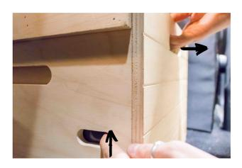
The drawers have a lock system, preventing them from opening when driving. To open the drawers, press down on the black plastic lock located on the side of the drawer, while pulling the drawer by the handle. Make sure to remove your finger when opening the drawer.
