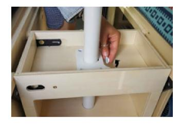
Screw the leg into the table and insert the lower part into the library box. Turn the tumb screw to tighten the leg and prevent the table from turning
