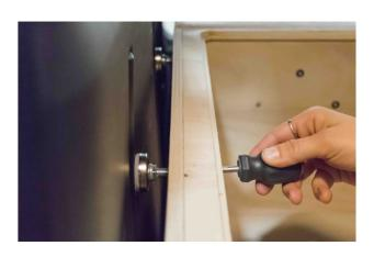
13. Using a flat screwdriver, adjust the leveling mounts on the side of the central module so it is well fixed against the walls of the vehicle so that the conversion kit is secured and won't move.
