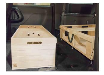
6. Insert the bench box into the vehicle. Align it with the central module.
