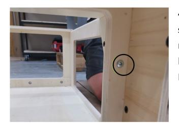
4. Fix the boxes together by affixing the screw on the interior side of the central module. The screw must be inserted in the box having no insert.
