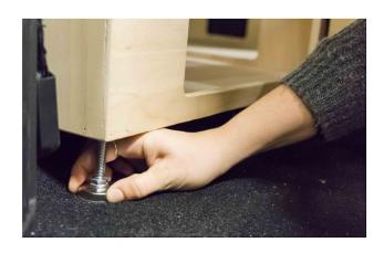
9. Adjust the height of the leveling pads so that the central module is fully supported on the ground.
