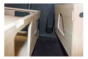
3.3 Insert the two rear boxes (sink drawer and burner drawer) in the fastening system of the central module.
