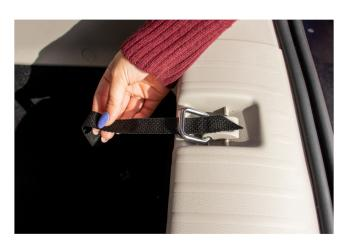
3.1 Insert the tip of the strap into the anchor.
