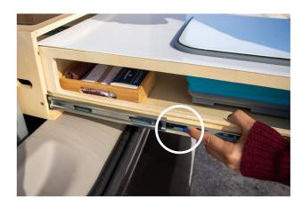
14. Open the kitchen drawer and squeeze the black latches simultaneously on each side of the drawer to open it an additional half inch.
