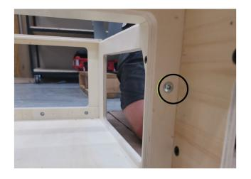
4. Fix the boxes together by affixing the screw on the interior side of the central module. The screw must be inserted in the box having no insert.
