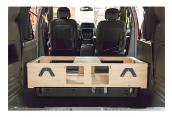
2. Insert the central module into the vehicle and place it in the center of the space.
