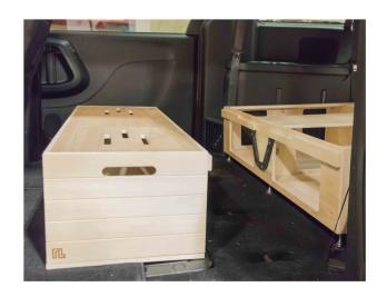
6. Insert the front bench into the vehicle. Align it with the central module.
