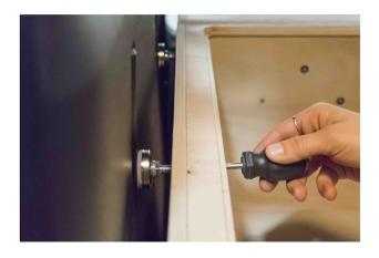
13. Using a flat screwdriver, turn the leveling pads until the central module is firmly seated against the walls of the car. In this way, the conversion set will not move and be secure.
