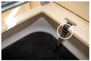
14.3 Tighten the strap well so that the drawer cannot move. Make sure the clip is underneath and not blocking the drawer from closing.
