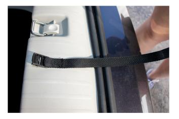
3. Install the drawer tie straps into the anchorage at the rear of the vehicle. Make sure it's the right way round.
