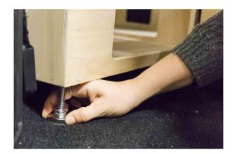
9. Adjust the height of the leveling pads so that the central box is fully resting on the ground and is level with the front box and the bookcase.
