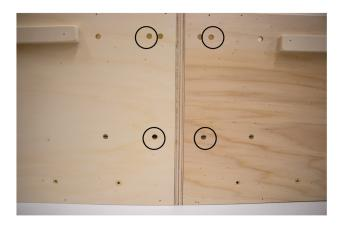
4. Attach the U-bracket to the center of the two boxes.
