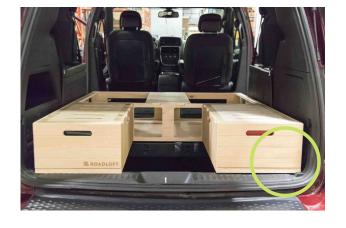
7. Make sure that the front of the rear boxes rests against the corner of the vehicle. Thereby, the central box will be found in its exact position. Take care to move the central unit AND the drawer units at the same time. Do not pull only on the drawer units to adjust the position.
