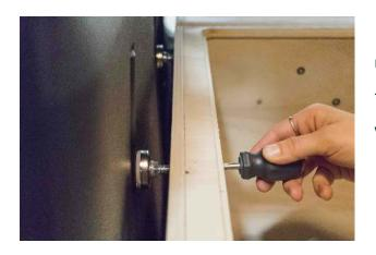
14. Using a flat screwdriver, turn the leveling pads until the central module is firmly seated against the walls of the car. In this way, the conversion set will not move and be secure.
