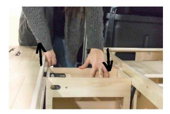
10. If necessary, slightly lift the front box to fully insert the bookcase.
