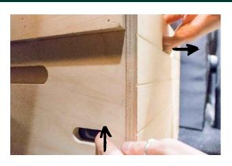
The drawers have a lock system, preventing them from opening when driving. To open the drawers, press down on the black plastic piece located on the side of the drawer, while pulling the drawer by the handle. Make sure to remove your finger when opening the drawer.
