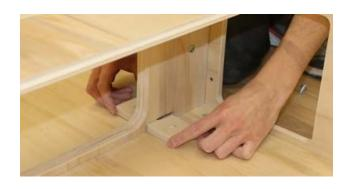
2.1 Insert the connector piece on each side so that the hole in the connector piece aligns with the box with a black insert.
