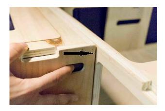
6. Lock out the caissons. To do this, slide the lock of the drawers towards the central box.
