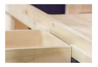
12. Make sure that the bookcase is correctly positioned: all the upper edges must be at the same level.
