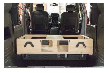
4. Insert the central housing into the vehicle and place it in the center of the space.
