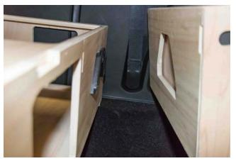
5. Insert the two rear boxes (sink drawer and burner drawer) in the fastening system of the central box.
